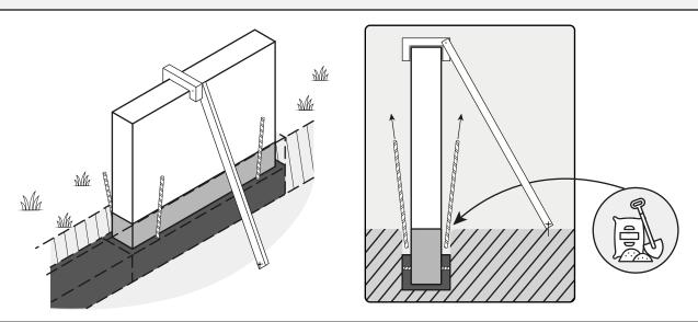
12. After the sand-cement mix has hardened in the foundation trench, fill the remaining 5 cm of the trench with a layer of decorative gravel.
