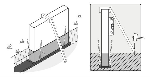
11. Fill the foundation trench evenly around the panel in layers, lightly compacting (tamping) the sand-cement mix to about 5 cm below the ground level around the foundation trench. During the filling process, monitor the vertical alignment of the panel.
